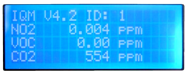
4-line x 20-character scrolling display shows data by parameter, value and unit in real-time
