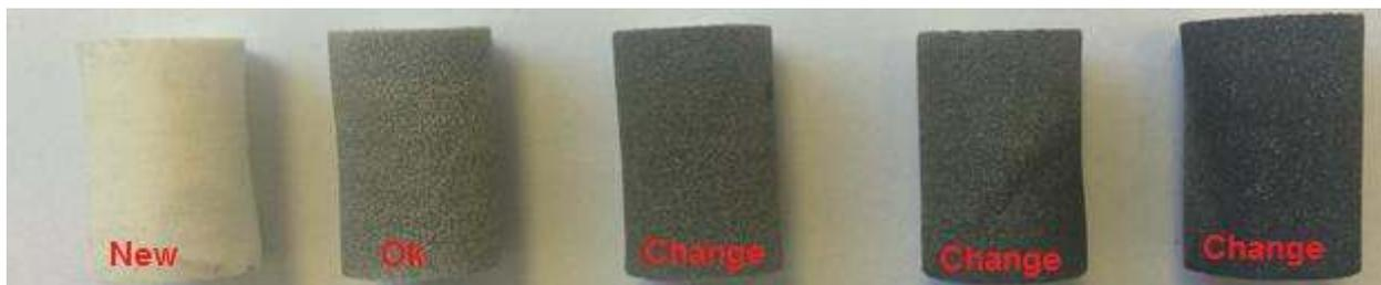
Figure 2. Examples of Dirty Particle Monitor filters, compared to a clean filter on the left.
