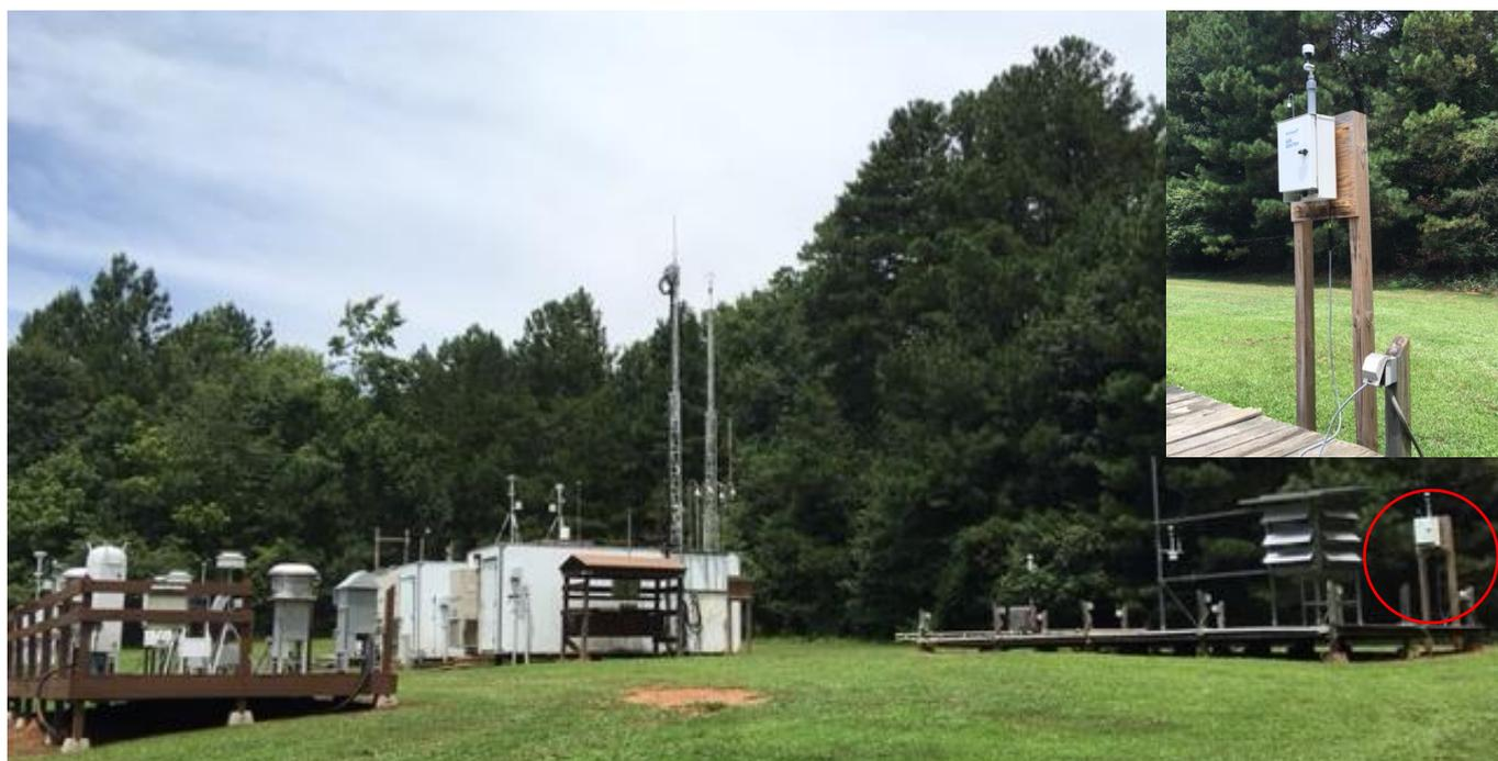
Aeroqual AQS1 is colocated with Federal Reference air monitors at the National Core (NCore) monitoring site at Decatur, South DeKalb, Georgia
