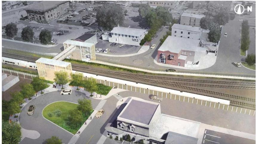
The LIRR Expansion Project improvements include a third track, new parking facilities and passenger rail stations, and elimination of seven street-level crossings.
