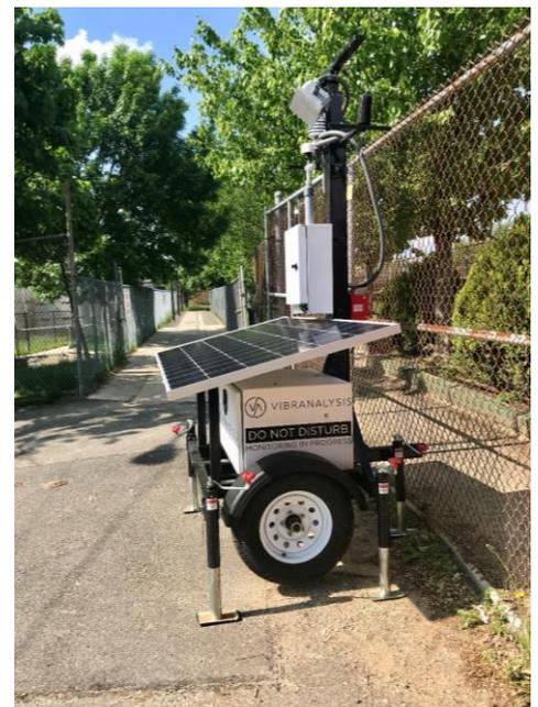
Vibranalysis conducted community air monitoring using 25 portable stations powered by Aeroqual AQS 1 along the LIRR Expansion Project in Nassau County, NY. The highly maneuverable systems included noise and weather sensors, cameras, telemetry, solar panel and batteries.
