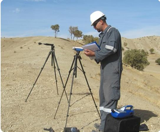
Such an extensive and diversified study meant the budgets were restricted for each discipline and respective equipment. The air quality component alone required measurement of five gases (H<sub>2</sub>S, SO<sub>2</sub>, O<sub>3</sub>, VOC and NO<sub>2</sub>) to establish the ambient air baseline.
