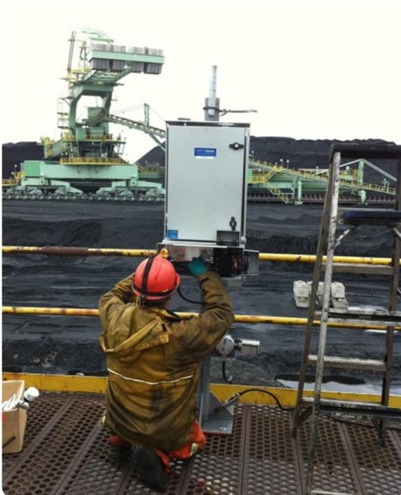
The two stations, located at different locations on and off the RTI site each contain a nephelometer for measuring  $PM_{10}$  particulates, a gas module for measuring carbon monoxide, fully integrated wind speed and wind direction sensors along with relative humidity and temperature sensors.
