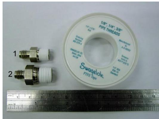
If your pressure regulator has a 1/8" Female NPT thread you should purchase part number SS-200-1-2 from Swagelok. This is fitting 1 in the above image.
