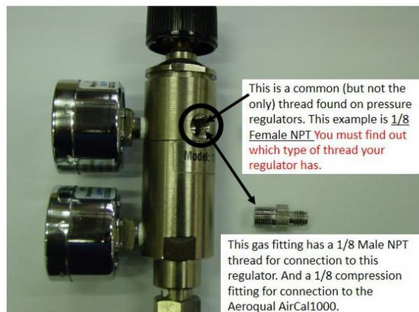
There are a number of possible thread types found on pressure regulators, but two common threads you will find on the outlet port of a pressure regulator are: 1/4 Female NPT or 1/8 Female NPT.
